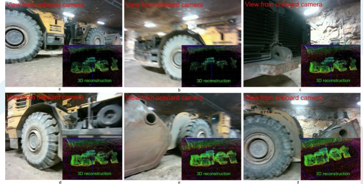
Video snapshots and 3D dimensional reconstruction of the environment based on an autonomous inspection scenario
